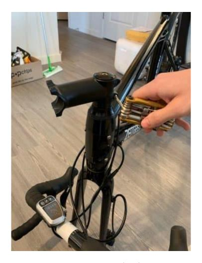
5. On the handlebar stem, loosen the Allen (hex) bolt with an Allen Wrench, reverse the stem 180 degrees into the forward position and tighten. Be sure the stem is on straight.
