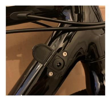
12. Plug the charger into the charging port located on the down tube and then into the wall outlet. The charger indicator light will turn green when fully charged.
