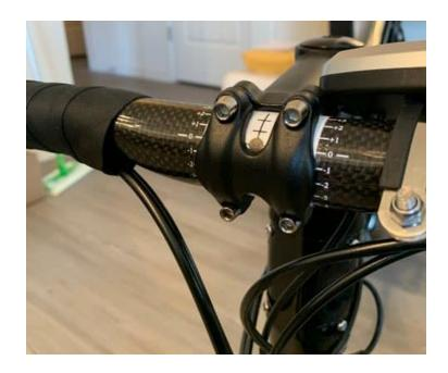
6. Get handlebar mount clamp and associated Allen heads from the plastic bag. Position handlebars as desired and tighten down with an Allen Wrench.
