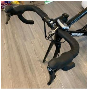
7. Adjust the handlebars to a comfortable position, and tighten Allen heads snugly. Tighten bolts in a X pattern for easiest tightening.
