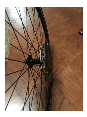
8a. Open the front wheel quick release lever. Remove locknut and spring. Slide quick release through axle, replace spring and locknut on shaft. Turn locknut only a few turns so it's loose for easy wheel installation.
