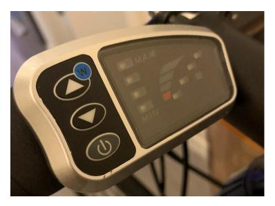
**Controlling the pedal assist strength:** Use the up and down arrows in the display shown above to increase or decrease the pedal assist. To ride without assist simply press the display power button. The assist will turn of above 28MPH as this is the maximum legal limit.
