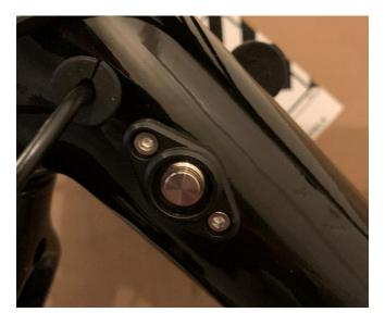
Step 2: Press the power button on the bottom left hand corner of the handlebar display show below.
